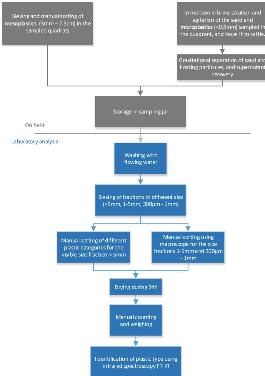
*Figure 4 : Block diagram of the meso- (5 mm- 2.5 cm) and microplastics (< 5 mm) sampling and analysis methodology. Plastic debris were collected on a quadrat area (0.25 m<sup>2</sup> area and 10 cm depth).*
