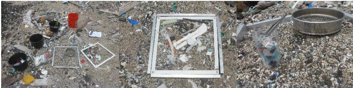
*Figure 2: Meso- and microplastics sampling on a quadrat (0.25 m<sup>2</sup> area and 10 cm depth), at Kamilo Point, Hawaii, on 30 June 2015 (F. Sciacca pictures).*
