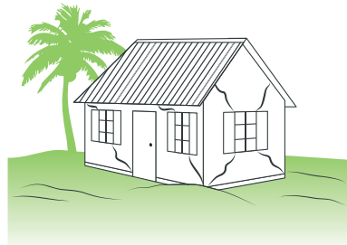
Figure 17: Cracks in solid walls (earthquake)
